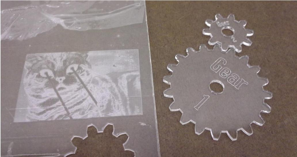
The Universal VLS6.60 laser can raster and vector based files.
