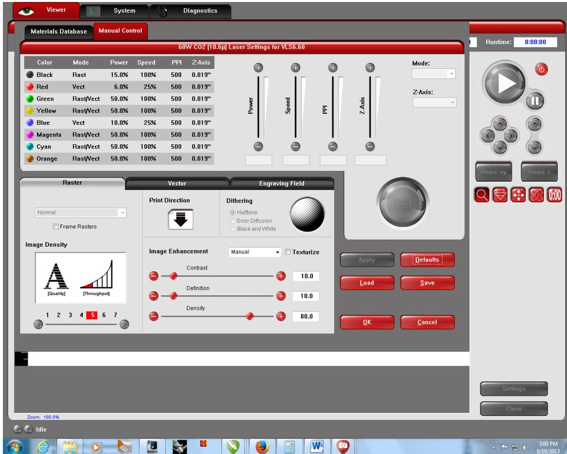
This screen let you set the laser power, speed, and material thickness. The settings for each path can be manually adjusted from this tab. Look at the various cut samples (on the wall in Fab Lab) to determine the cut depth and speed appropriate for the material that you are cutting.
