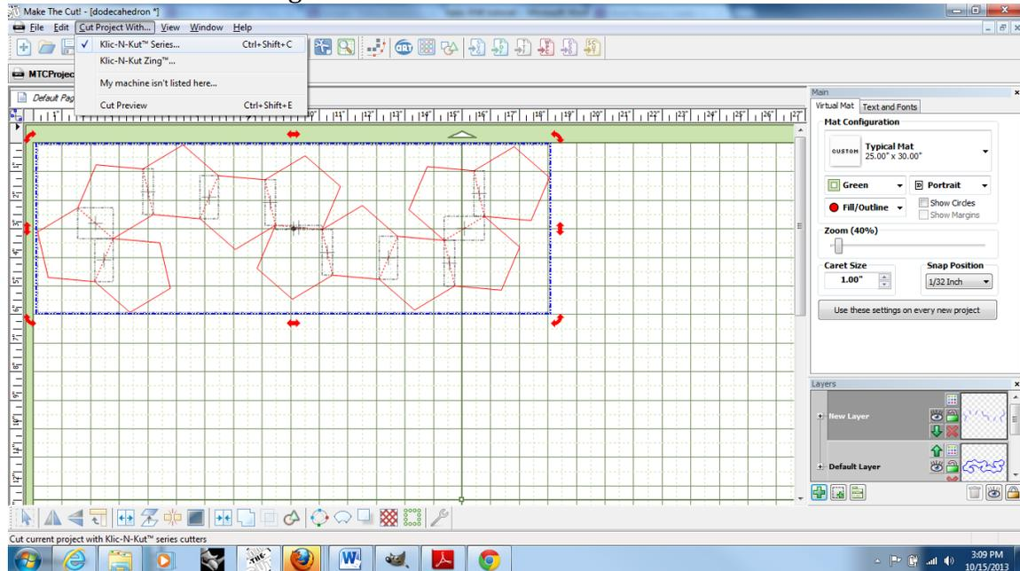
To cut the design go to **Cut Project With...>Klic-N-Kut Series** or **Ctrl+Shift+C**
