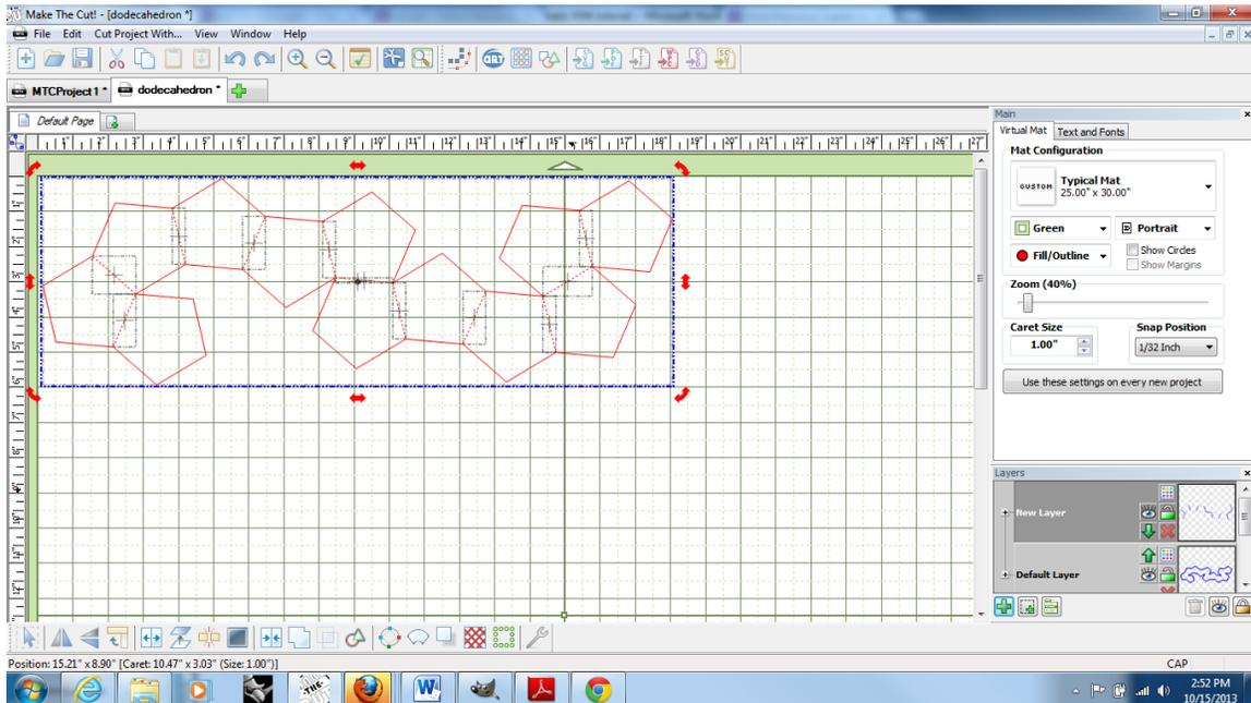
In knife point mode the cut will always start from the bottom right corner of the design regardless of placement on the virtual mat. It is important to make sure that the design will fit on the sheet of material it is being cut from. Use rulers at the top and left ensure the design is the correct size.
